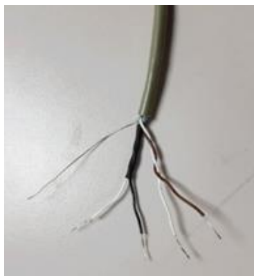
Figure 7 Modbus Connector Cable Part - Binder 99-9210-00-04 (Front View)
