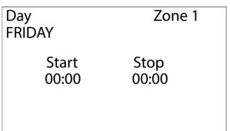
This mask is used to modify the day of the week and the times of zone 1 (see the Zone diagram).
