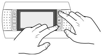
When the desired menu is seen press the key 🕐 to enter the menu. Press the key
