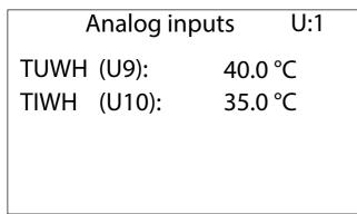
— TUWH (U9): condenser water outlet temperature
