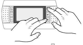
When the desired parameter is seen press the key  $\checkmark$  to enter the parameter. To exit the parameter and return to the parameter selection mode press the key  $\boxed{\epsilon_{ex}}$ .
