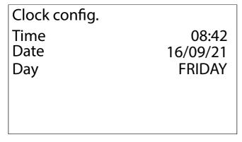
This mask is used to display and modify the time, date and day of the week parameters.
