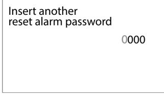
Entering a new password for gas alarm reset.
