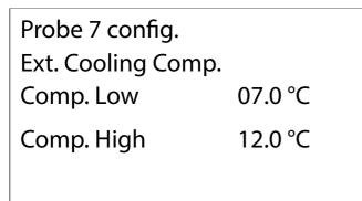
Multifunction input enabled with setpoint compensation with temperature probe function (MASTER ONLY)
