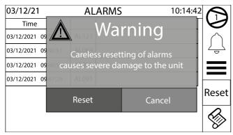
To reset the alarms, simply press the Reset key.
