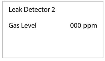
Concentration of flammable gas detected by sensor 2.
