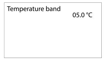
Proportional band for the adjustment of the work thermostat (MASTER ONLY).
