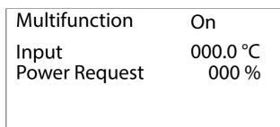
Multifunction input enabled for cooling capacity request
