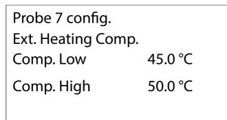
Multifunction input enabled with setpoint compensation with temperature probe function (MASTER ONLY)
