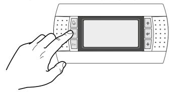
Once in the menu selection mode it is possible to move between menus using the arrow keys: the key (\*) to move to the previous menu, and the key (\*) to move to the next menu:
