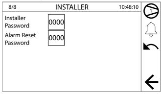
— Entering a new password for gas alarm reset.
