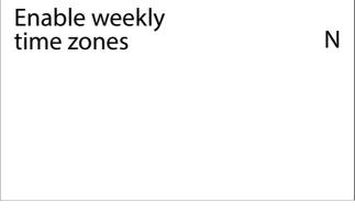
This mask is used to enable the weekly time band timer (Y = enabled, N = disabled).
