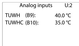
— TUWH (U9): condenser water outlet temperature
