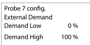
Multifunction input enabled with external power request function (MASTER ONLY)
