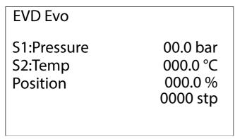
This mask is used to view the pressure, temperature and position of valve 1 and valve 2.
