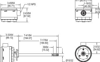
The Series AVLV Air Velocity Transmitter quickly and accurately measures air velocity or volumetric flow in imperial or metric units. Simultaneous current and voltage outputs on all models provide universal inputs to monitoring equipment while the output range, units, and 0-5/10 VDC output can be configured via local DIP switches. The optional integral display, or the portable remote tool, provide a convenient way to local monitor process values and configure the unit.
