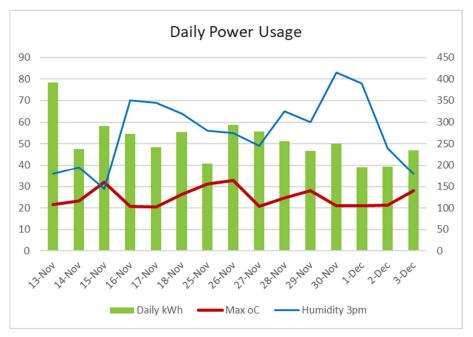
The above data indicates a reduction in energy usage between the pre-treatment (13 Nov – 18 Nov) and post treatment (25 Nov – 3 Dec) periods (coating applied 22<sup>nd</sup> November) even though the operating conditions might be considered to be slightly more onerous in the post treatment period – slightly higher temperatures and humidity.
