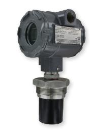
The **Series ULT Ultrasonic Level Transmitter** provides non-contact measurement of liquid levels in an explosion-proof body. It is capable of measuring up to 32.8' (10 m) with a PVDF sensor and 4 to 20 mA output.
