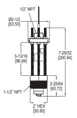
The Series PFT Paddlewheel Flow Sensor is used to monitor liquid flow rates in pipes from 1-1/2 to 40" and is available in brass or 316 SS body. The unit outputs a frequency proportional pulsed or 4-20 mA output. The pulse models are a square wave output signal with frequency proportional to the flow velocity and the 4-20 mA models have a linear output of the velocity with 4 mA equal to 0 ft/s and 20 mA equal to 25 ft/s.
