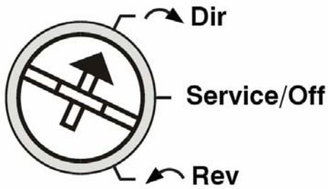
Fig. 3. Function selection switch
