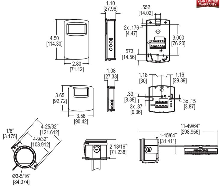
The Series CDTR Carbon Dioxide, Relative Humidity and Temperature Transmitters reduce the number of sensors mounted on a wall or in a duct. By combining CO<sub>2</sub>, RH, and temperature in one device, system integrators are able to reduce installation time while lowering material cost at the same time.
